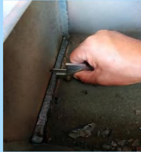
焊缝检查 weld inspection
